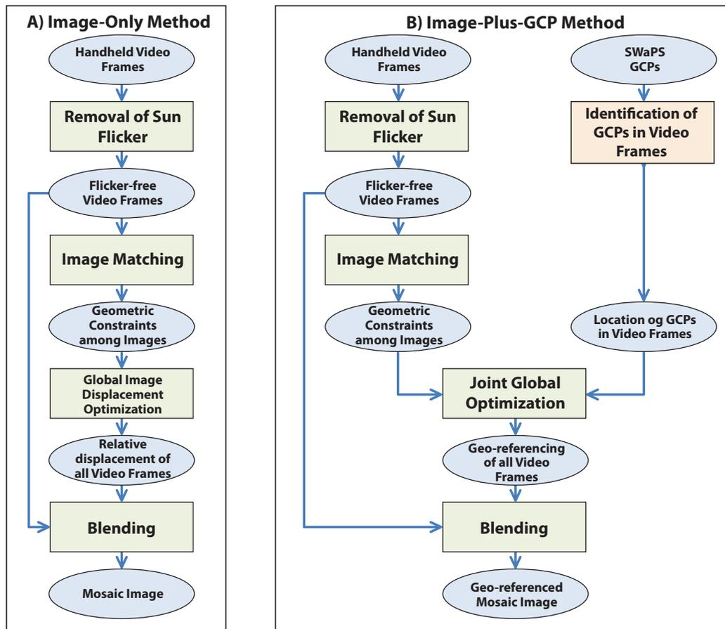
**Fig. 2.** Flow charts illustrating the data (ellipses) and the processing steps (rectangles) for the image-only method (A) and the image-plus-GCP method (B) of mosaic creation. Fully automated processing steps are in light green. The only step requiring user intervention is in light red (identification of ground control points in video frames). The primary difference between the algorithms is in the cost function minimized in the global optimization step.
